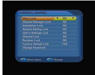
Installation Lock: To lock the installation menu to prevent unauthorized adjusting of Installation.
